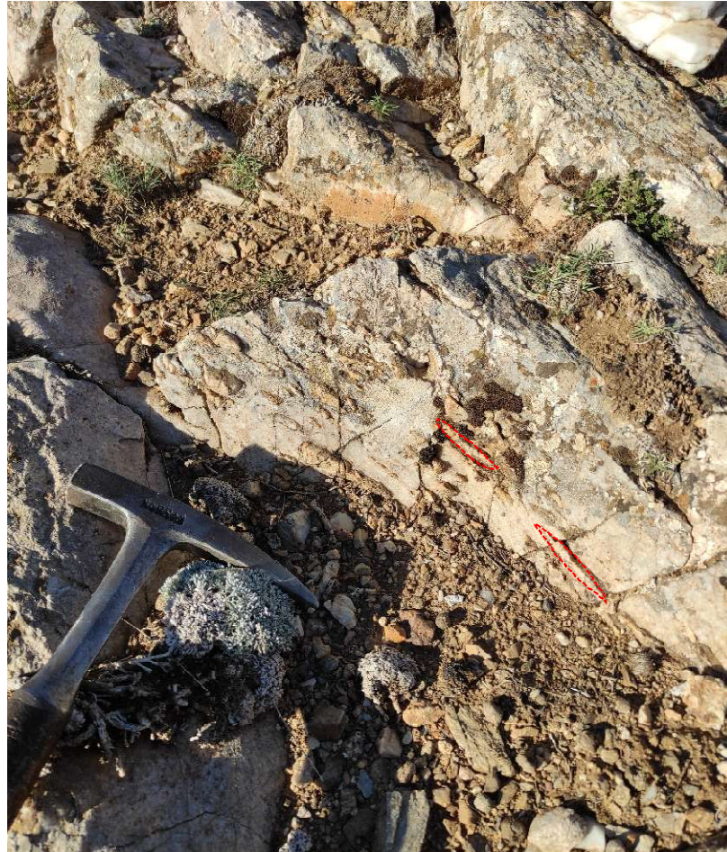
Figure 2.8. Quartz lens formed along the foliation planes in marble (37.933073, 34.843609).
