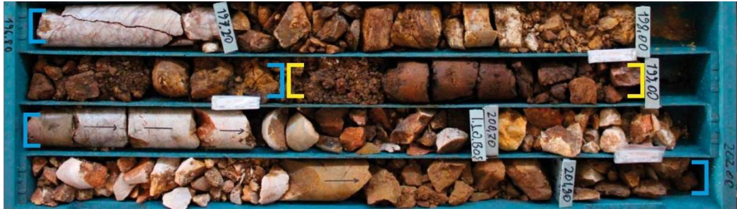
Figure 2.20. Gossans (interval within yellow brackets) in marble (interval within blue brackets).
