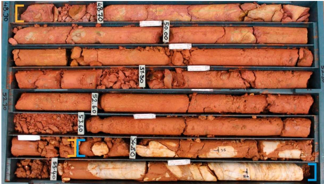
Figure 2.19. Highly-oxidized cataclastic breccias (intervals within orange brackets) and underlying MKBX (intervals within blue brackets) in a drillhole.
